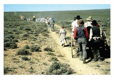
The handcarts were modeled after carts used by street sweepers and were made almost entirely of wood. They were generally six to seven feet long, wide enough to span a narrow wagon track, and could be alternately pushed or pulled. The small boxes affixed to the carts were three to four feet long and eight inches (203 mm) high. They could carry about 500 pounds, most of this weight consisting of trail provisions and a few personal possessions.
